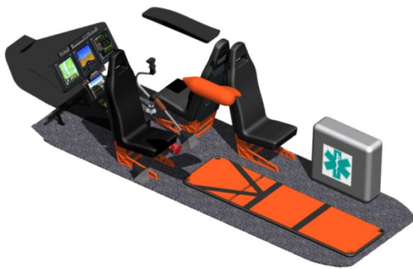
Figure 16.8 Cabin layout for coast guard rescue mission
