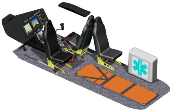
Figure 16.10 Cabin layout for EMS mission
