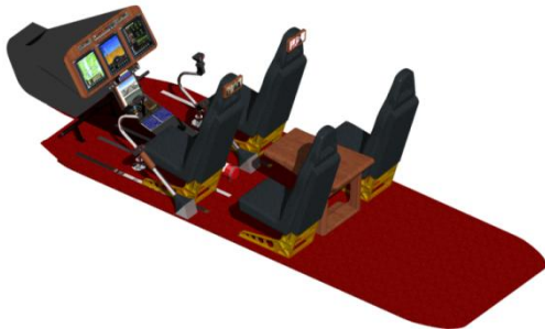
Figure 16.4 Cabin layout for corporate/VIP mission
